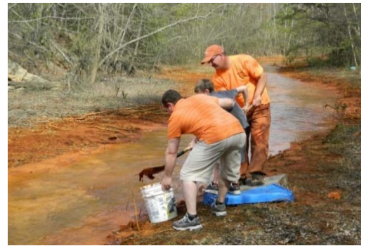
PHOTO CREDIT: EPCAMR. PENNSYLVANIA STUDENTS COLLECT IRON OXIDE FROM ACID MINE DRAINAGE TO MAKE PIGMENTS.
